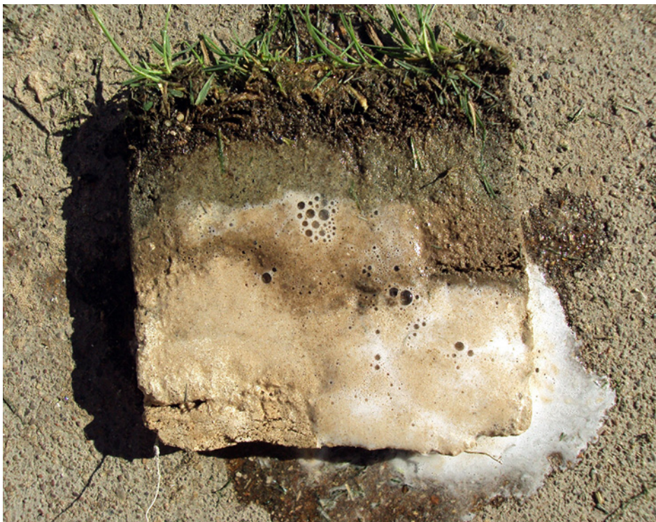
When acid is placed on a soil containing appreciable calcium carbonate, the soil fizzes in the form of carbon dioxide gas bubbles.
