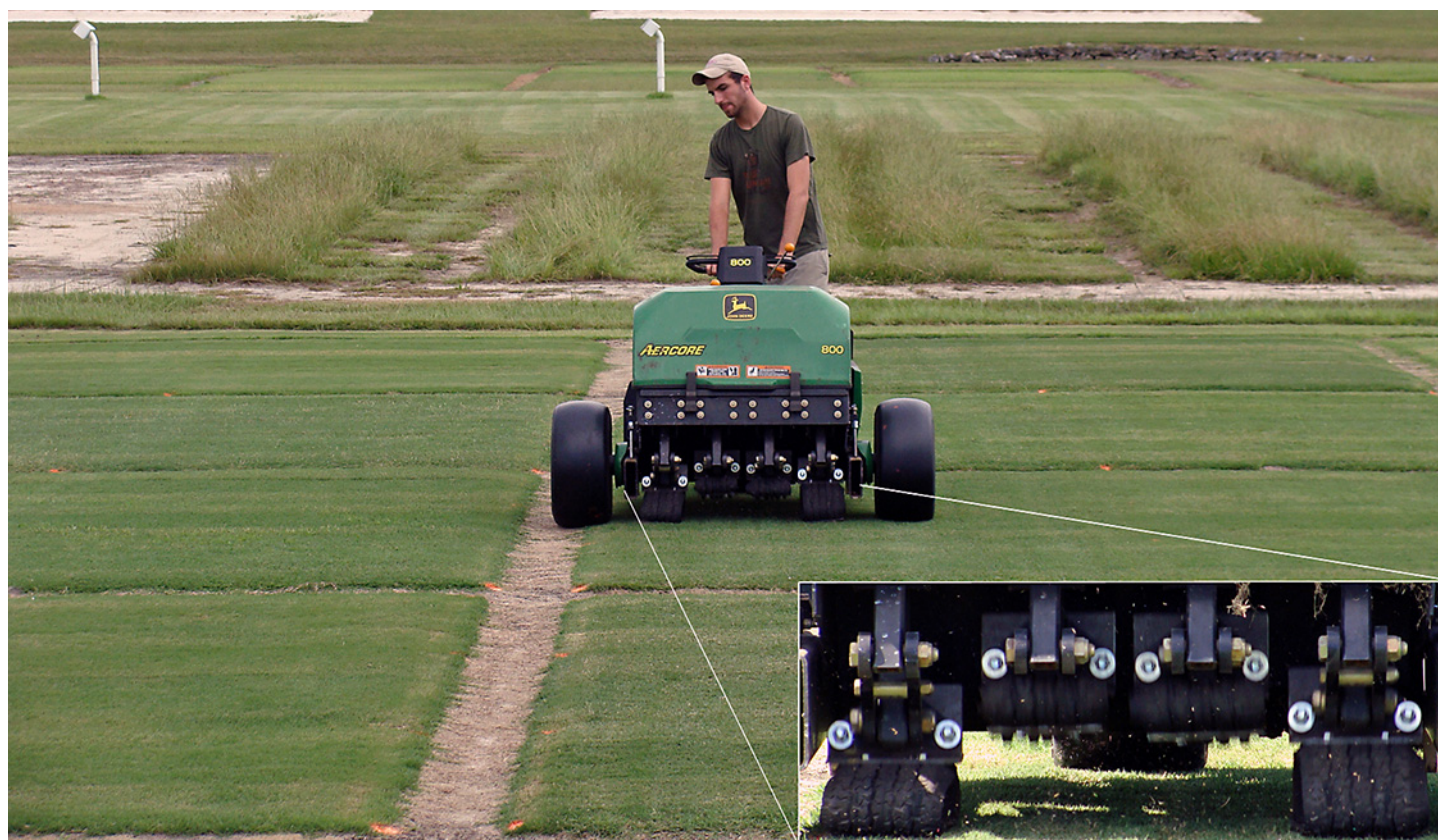
A modified Cady traffic simulator was used to apply traffic once per week during the study period.
