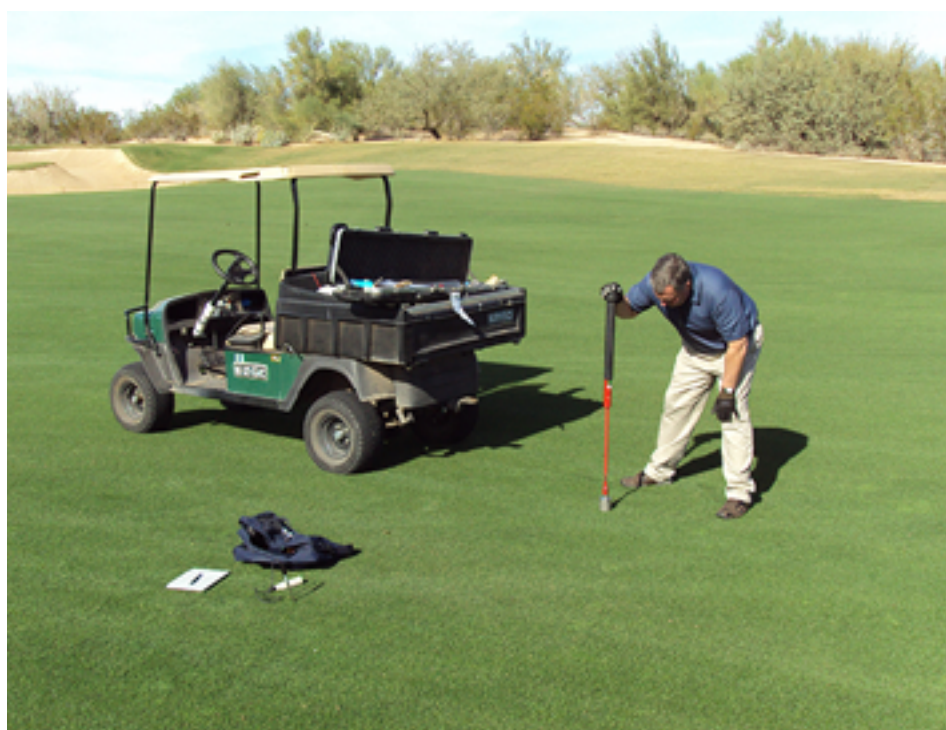
Dr. Norm Hummel collects a soil core for physical analysis. An AMS Soil-Core Sampler was used to collect 8- to 12-inches-deep soil-core samples from fairways. The sampling equipment was broken multiple times when driving the device into these hard, compacted soils.
