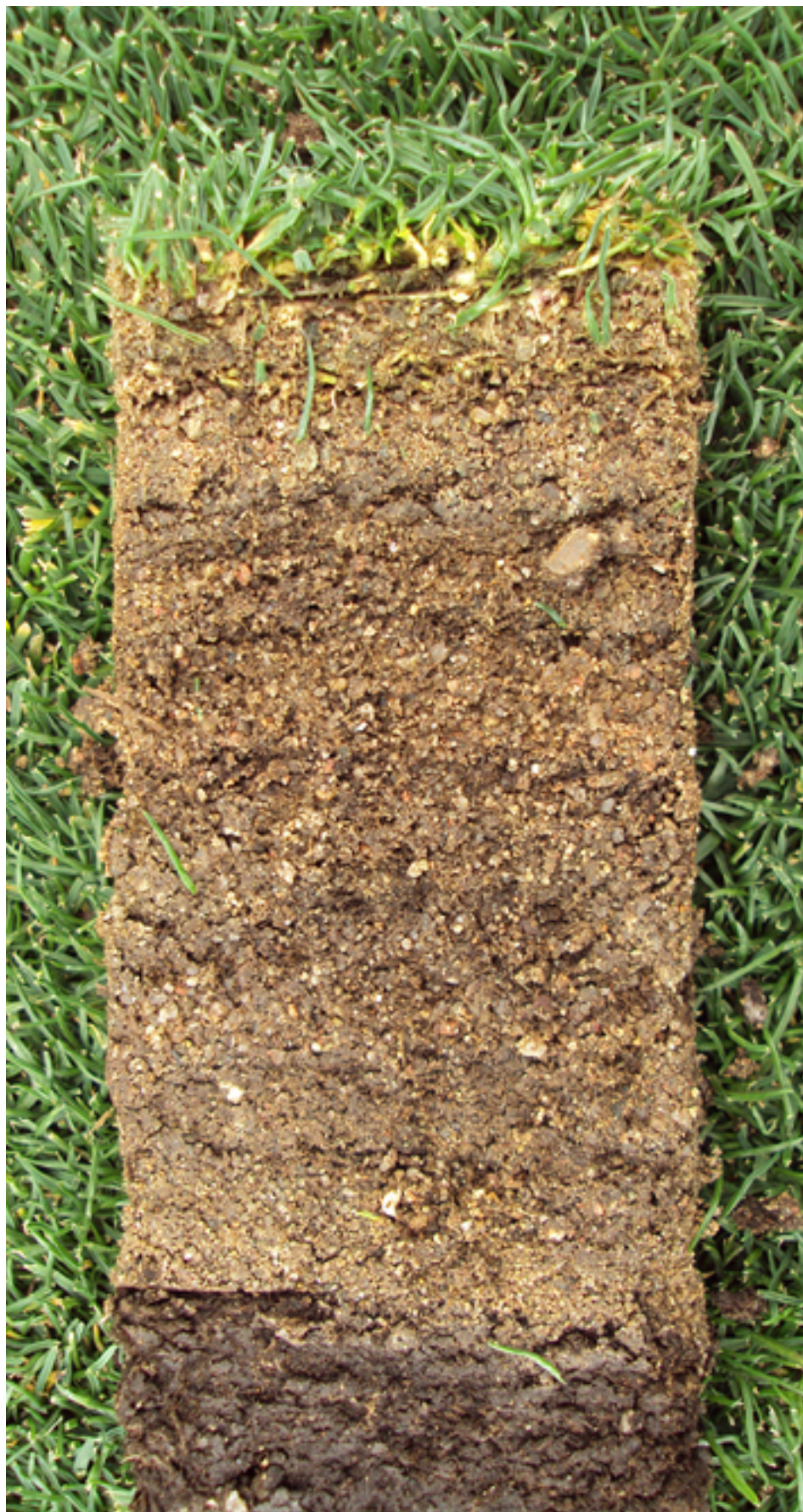
Over 6 inches of sand has been applied to these fairways, yielding firm surfaces and excellent turfgrass quality.
