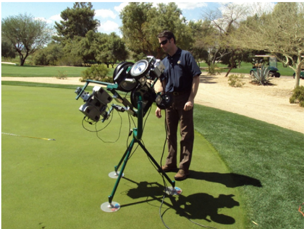
A modified baseball pitching machine was used to fire golf balls into the turf with a range of speeds, spins, and angles.
