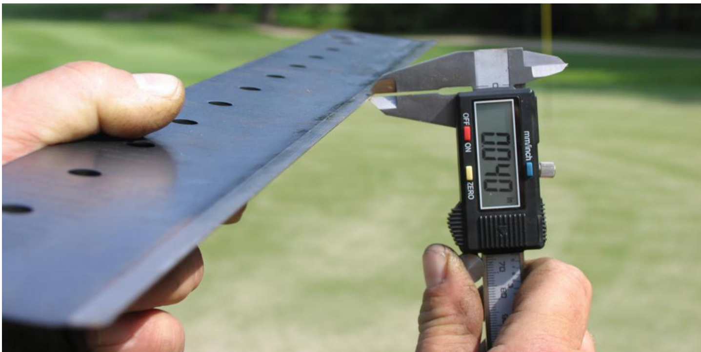
At very low effective mowing heights, use the thinnest bedknife available or grind the bedknife to a thinner thickness to provide enough clearance between the bottom of the bedknife and the ground. Source: Rodney Lingle.
