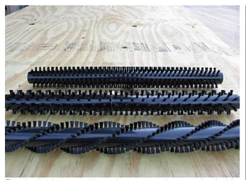
These brush styles are gear-driven and counter-rotate when mounted on the John Deere walking greens mowers. The spiral version in the foreground is not nearly as aggressive as the brush (top) designed by Rodney Lingle, superintendent at Memphis Country Club.
