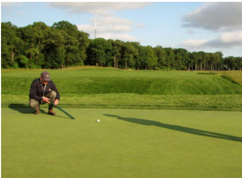
USGA agronomists measure green speed using the USGA Stimpmeter at least twice per day during professional and amateur national championships.
