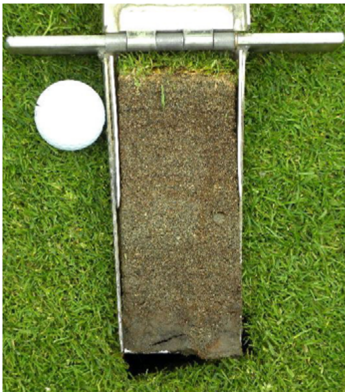
Figure 6: When aeration and topdressing programs properly dilute thatch accumulation, a rootzone free of organic layers is achieved. This soil profile exhibits excellent thatch management and blending of the new rootzone (sand topdressing and organic matter accumulation) with the sand-based construction mixture below.
