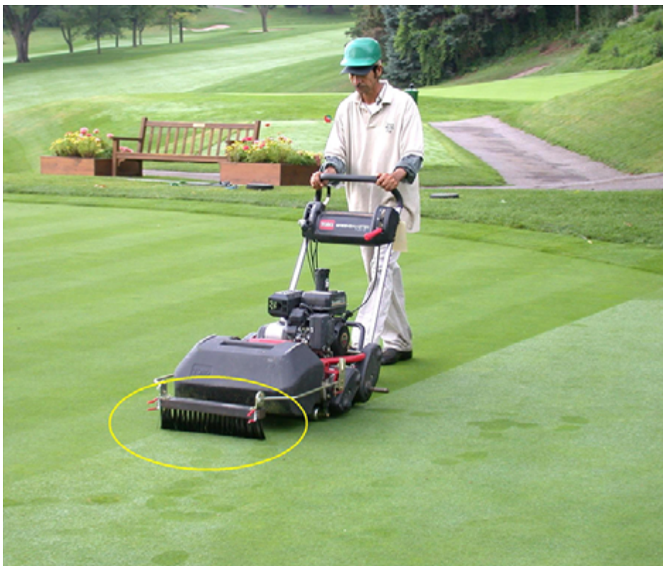
Some pictures speak for themselves. Want to make a point about motorized carts damaging soft, wet fairways? The image of muddy tire tracks says it all. In contrast, you may want to highlight more technical images with arrows or circles to make sure you and the audience are on the same page. Want to brag about how well the new brushes on walking greens mowers are standing up the turf for a cleaner cut? Be sure to highlight the brushes in the image to focus the reader's attention.
