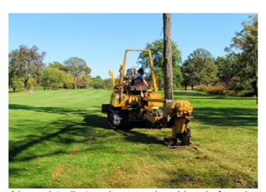
A heavy-duty vibratory plow can make quick work of severing tree roots without causing significant damage to turf. A rolling operation over the plow slit will make most surface disruption disappear. Be sure to locate and mark irrigation and underground utilities prior to root pruning operations.
