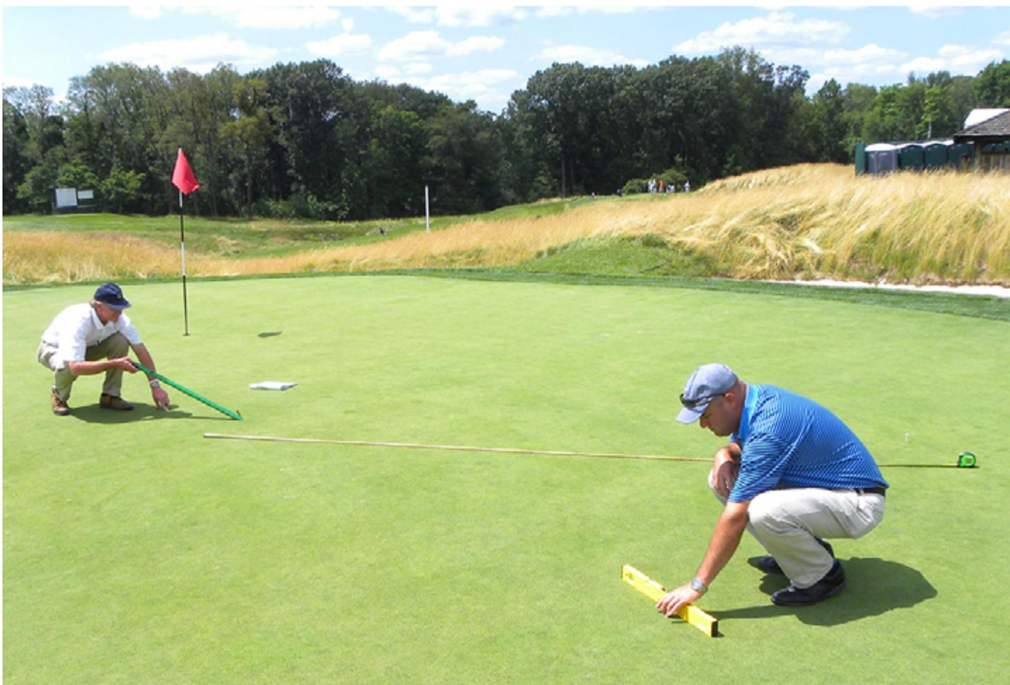
Various tools are available for use by golf facilities in setting realistic green speeds. In this photo, a Stimpmeter® and digital level are used to determine green speed and hole locations.
