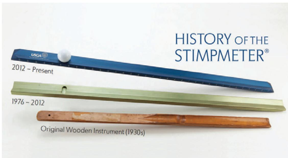
*From its humble beginning in the 1930s to the recently redesigned USGA Stimpmeter® in 2012, the readings that this simple device provides have single handedly become the barometer for evaluating putting greens. Focusing only on green speed, however, ignores other characteristics important to playability and putting surface quality, such as surface uniformity, trueness of ball roll and firmness.*
