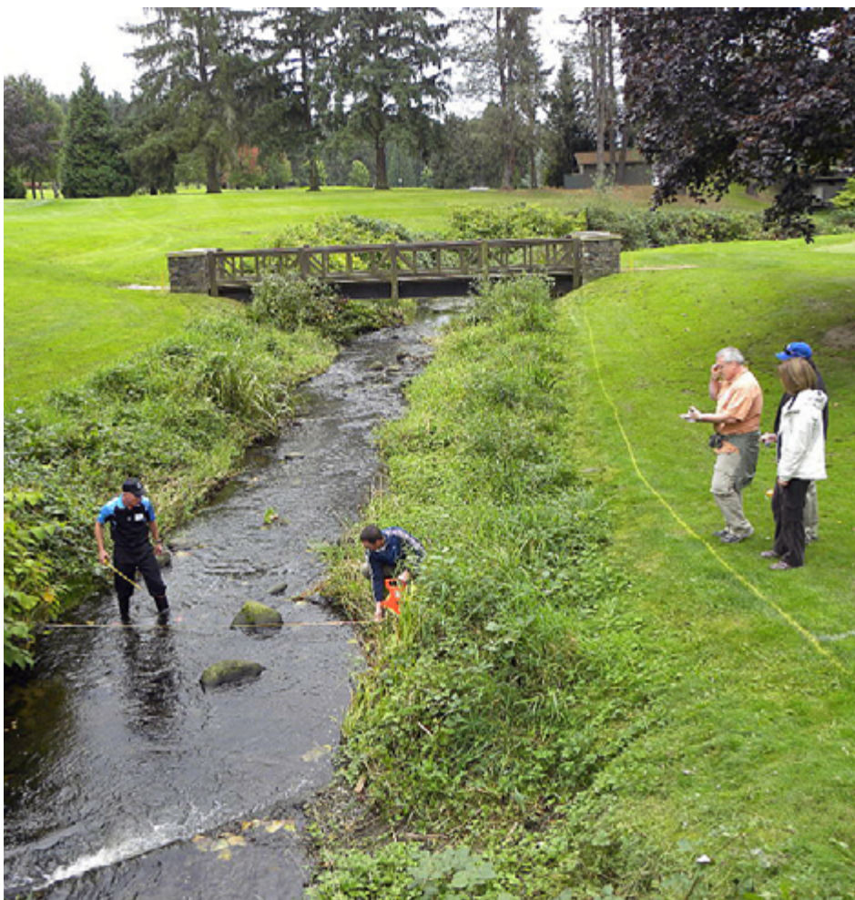
Steve Kealy, Superintendent at Glendale C.C., helps measure stream dimensions for determining water flow measurements.
