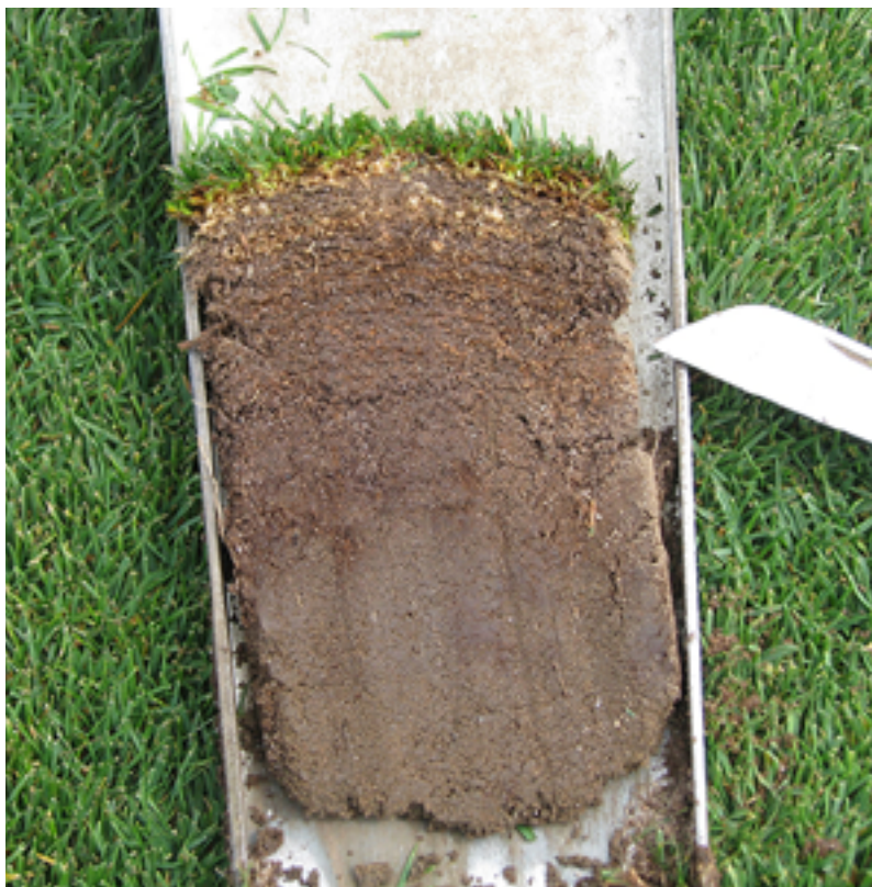
Examine soils closely to see if they require modification. Expansion areas often have higher thatch levels that must be reduced before greens can be expanded successfully.
