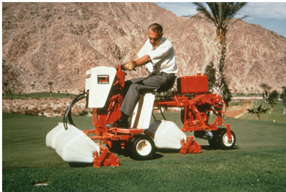
The 1968 Greens King. The original triplex putting green mower was developed in 1968 by Jacobsen® and named the "Greens King." The instant success earned recognition from Golf Digest in 2010 as one of their "Top 60 Innovations of Golf's Modern Era." (Photo courtesy of Jacobsen®)
