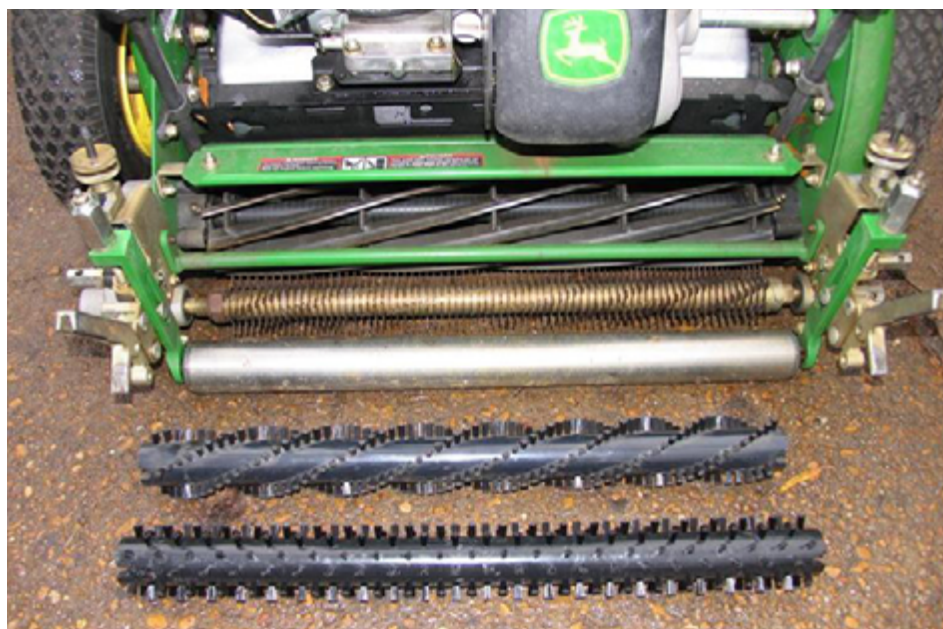
Innovative brushes and turf groomer attachments are available on triplexes and allow two operations to happen when mowing. New counter rotation of these attachments preserves reel and bedknife sharpness.
