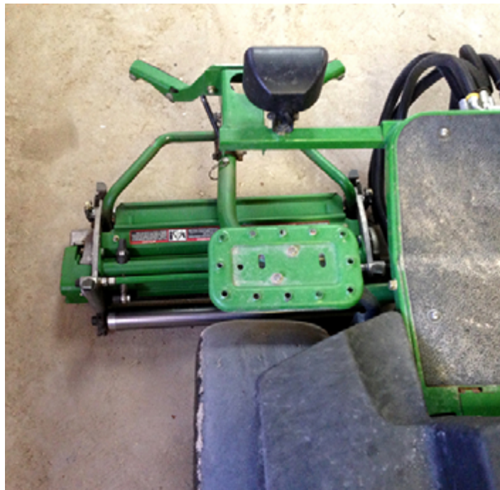
Offset cutting units from the center line of the triplex machine are a new design feature to counter the “triplex ring.” The offset feature is easily observed in these two views of the front reel units. Alternating the cutting direction when making the cleanup pass will ensure the tires will not follow the same path while mowing the green perimeter areas.
