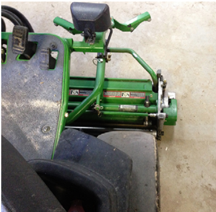
Offset cutting units from the center line of the triplex machine are a new design feature to counter the “triplex ring.” The offset feature is easily observed in these two views of the front reel units. Alternating the cutting direction when making the cleanup pass will ensure the tires will not follow the same path while mowing the green perimeter areas.
