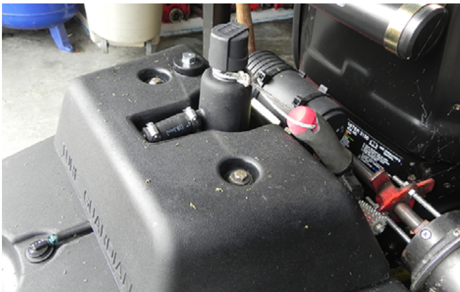
Hydraulic alarm systems signal to the mower operator when hydraulic leakage happens. This new advancement helps minimize turf injury.
