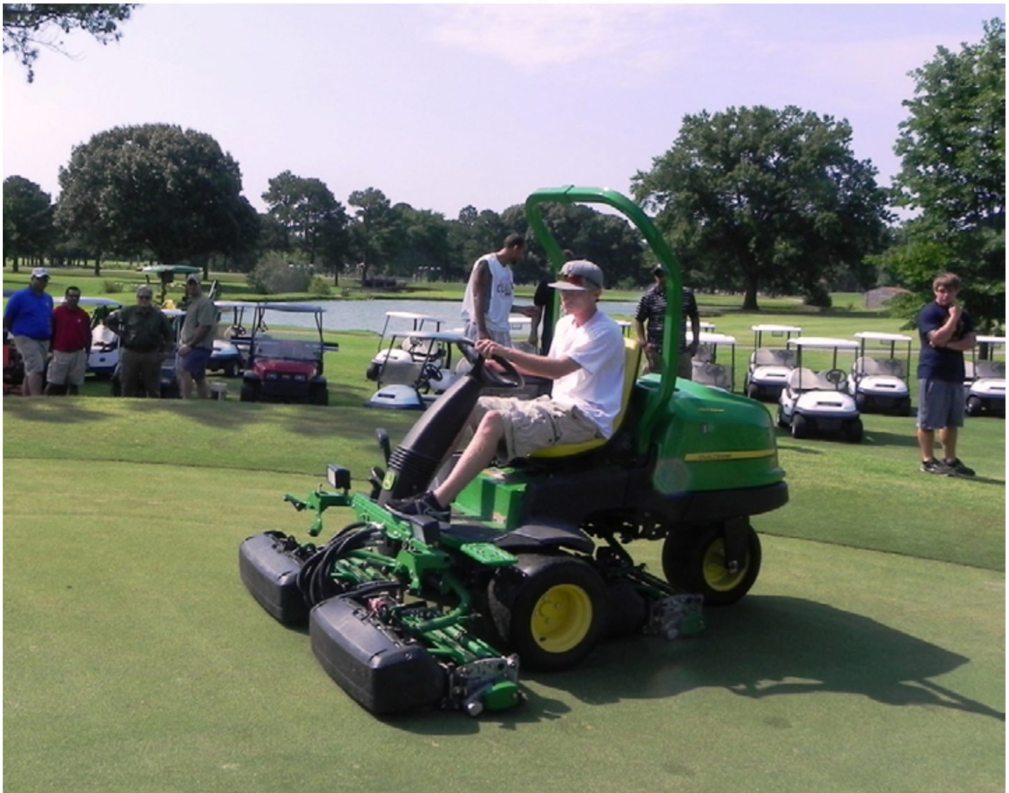
Triplex mowers are now essentially built around the identical cutting units as hand mowers. New hybrid and electric models reduce fuel costs and limit issues with hydraulic leaks.
