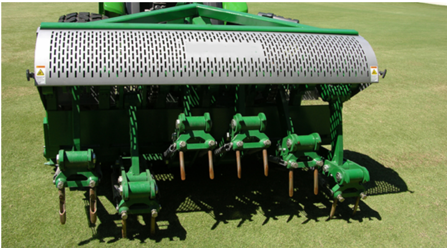
Solid-tine aeration provides relief from soil compaction in a quick and efficient manner with minimal disturbance.
