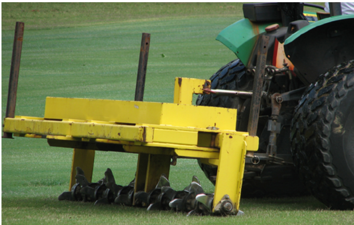
The heavy-duty slicer is an excellent tool to quickly alleviate water runoff issues associated with compacted soils. The slicing blades penetrate 6-8 inches into the rootzone and cause minimal surface disruption.
