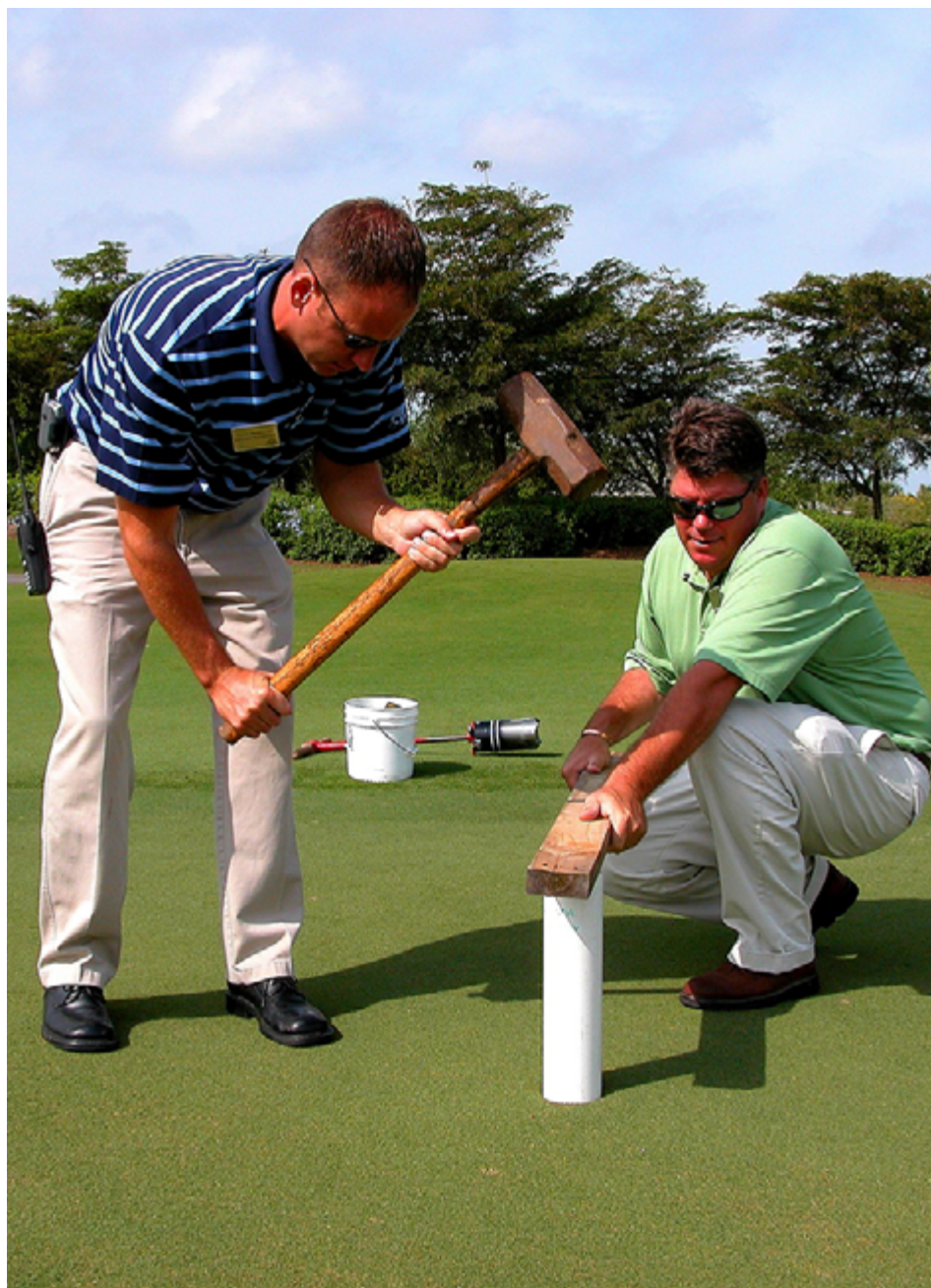
Undisturbed core analysis can determine important soil physical properties and whether soils drain adequately.
