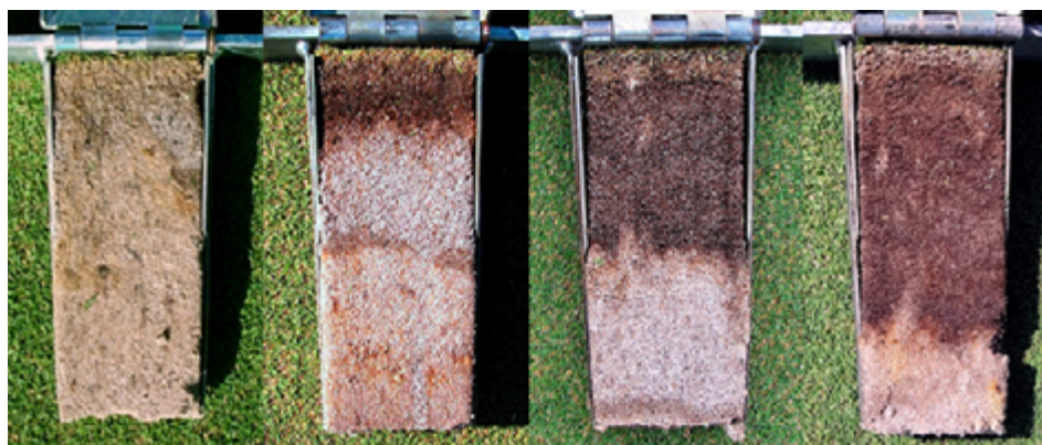
Organic matter accumulates at an accelerated pace on Florida putting greens, and this can negatively impact drainage and turfgrass rooting. To show how rootzones change with time, from left to right are soil profiles removed from the same putting green (renovated in 2001) in 2001, 2003, 2008, and 2012, respectively.
