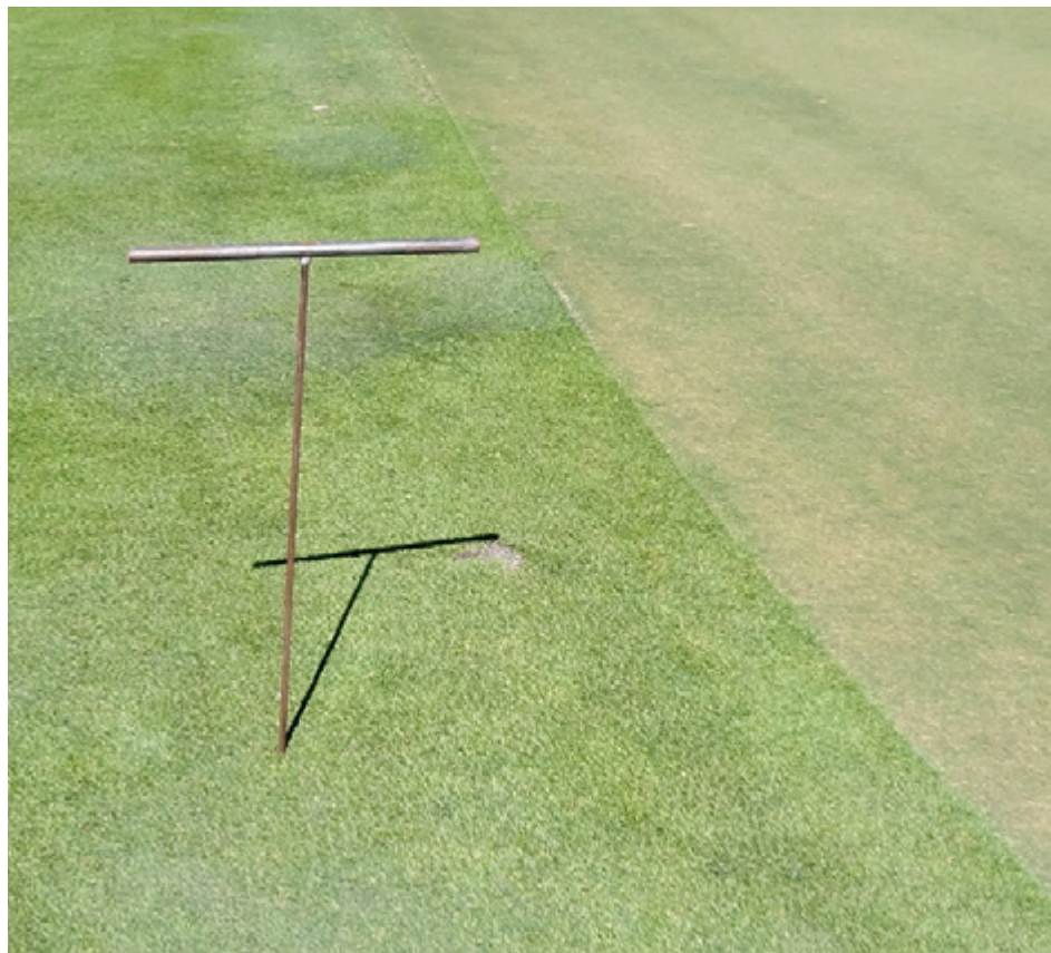
By locating the underlying gravel layer used to construct putting greens, irrigation probes can help determine how much of the surrounding grass has encroached onto putting greens. In this case, the current putting green perimeter has moved several feet away from its original location.
