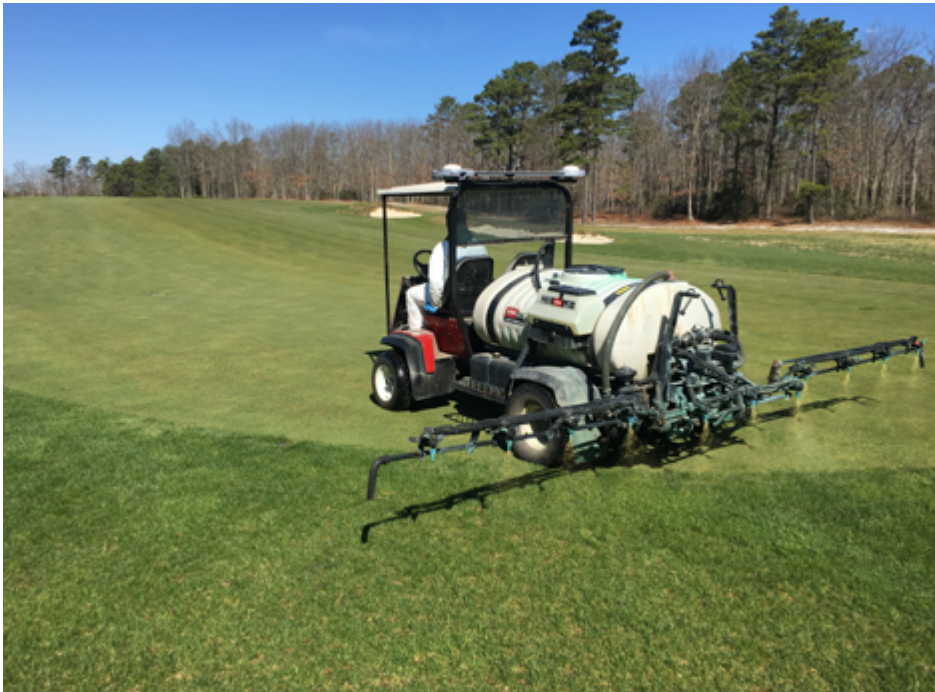
Spraying equipment that utilizes GPS technology can improve accuracy and decrease product use.
