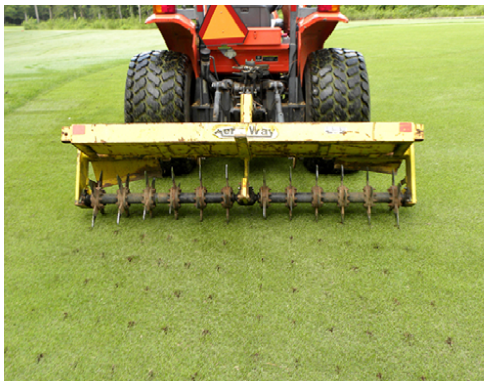
Aeration is an important water-conservation technique because it helps prevent the loss of surface water as runoff.
