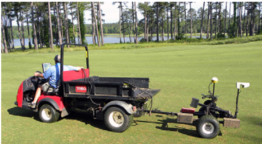
The first component of Precision Turf Management is to understand the components of the golf course property. A portable mobile mapping system is the first step conducted to map the property and to collect data and identify different soil types on the golf course.
