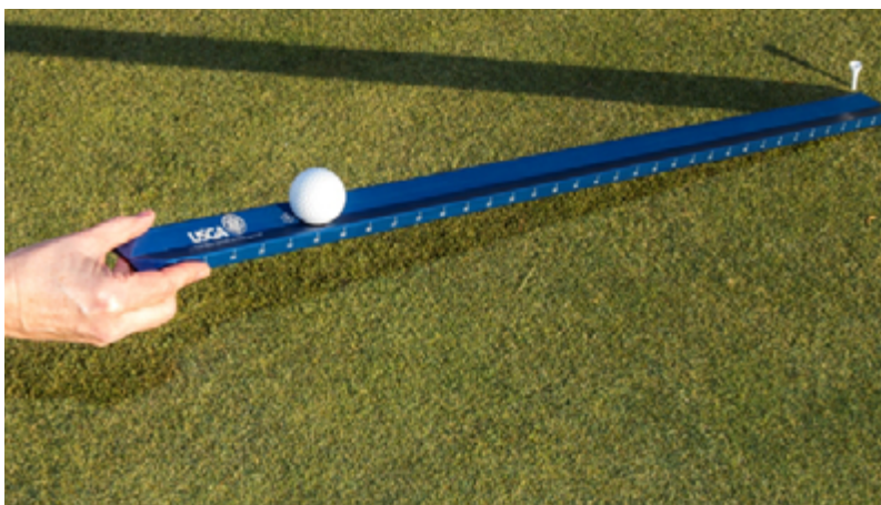
The USGA Stimpmeter measures green speed and provides valuable information to assist golf course superintendents in making day-to-day management decisions.
