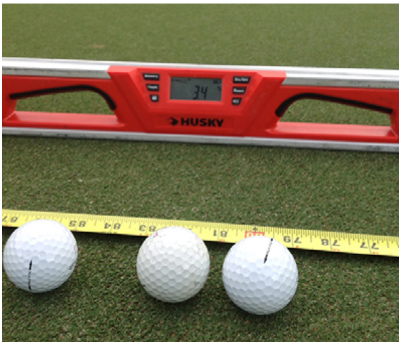
A digital level provides a precise measurement of the slope around a hole location.
