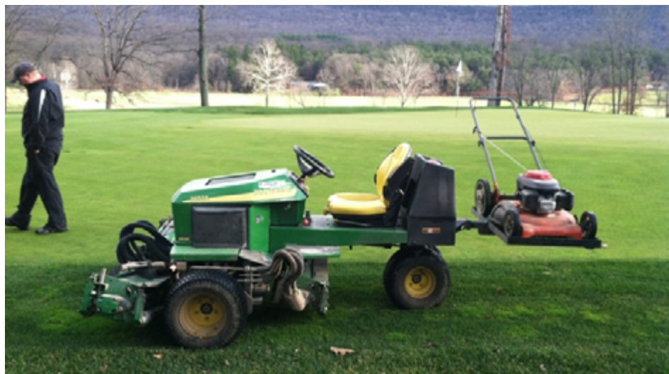
Superintendents are constantly challenged to come up with efficient ways of meeting golfer expectations while staying within budget. Combining maintenance tasks can improve efficiency, as in this photo where a rotary push mower is transported on the back of a triplex unit and the employee performs both mowing duties.
