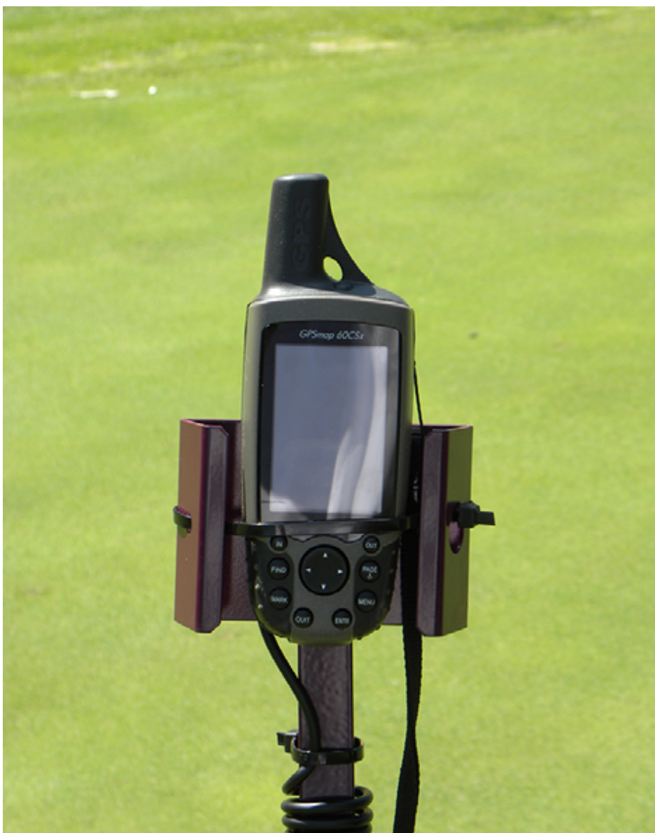
A GPS receiver can be integrated with the Field Scout moisture probe to produce accurate maps of putting greens and spatial variability across a putting green.
