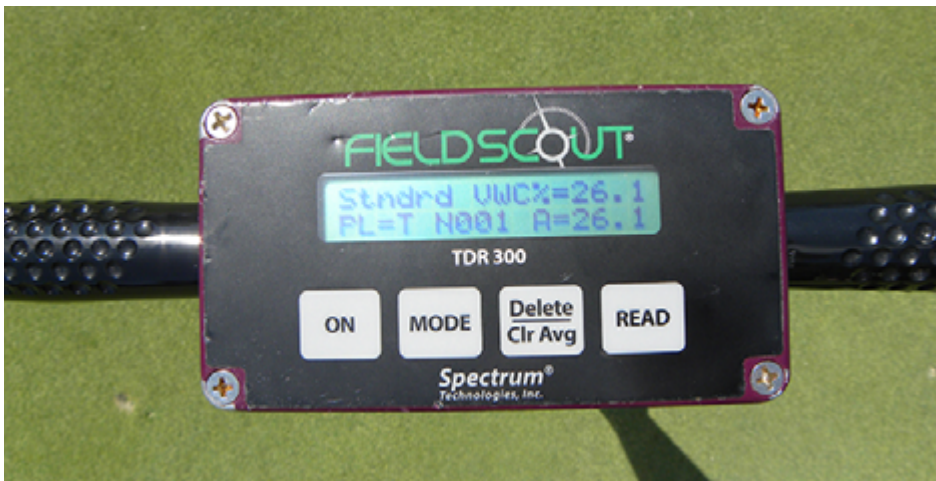
Expressed in percentage volumetric water content, the Field Scout moisture probe is easy to use and to read the results.
