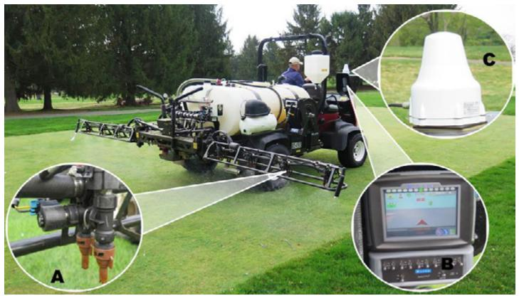
GPS-equipped sprayers include individual nozzle control solenoids (A) that automatically turn on and off, a display console (B) that shows application areas, and an antenna (C) that receives data from satellites.
