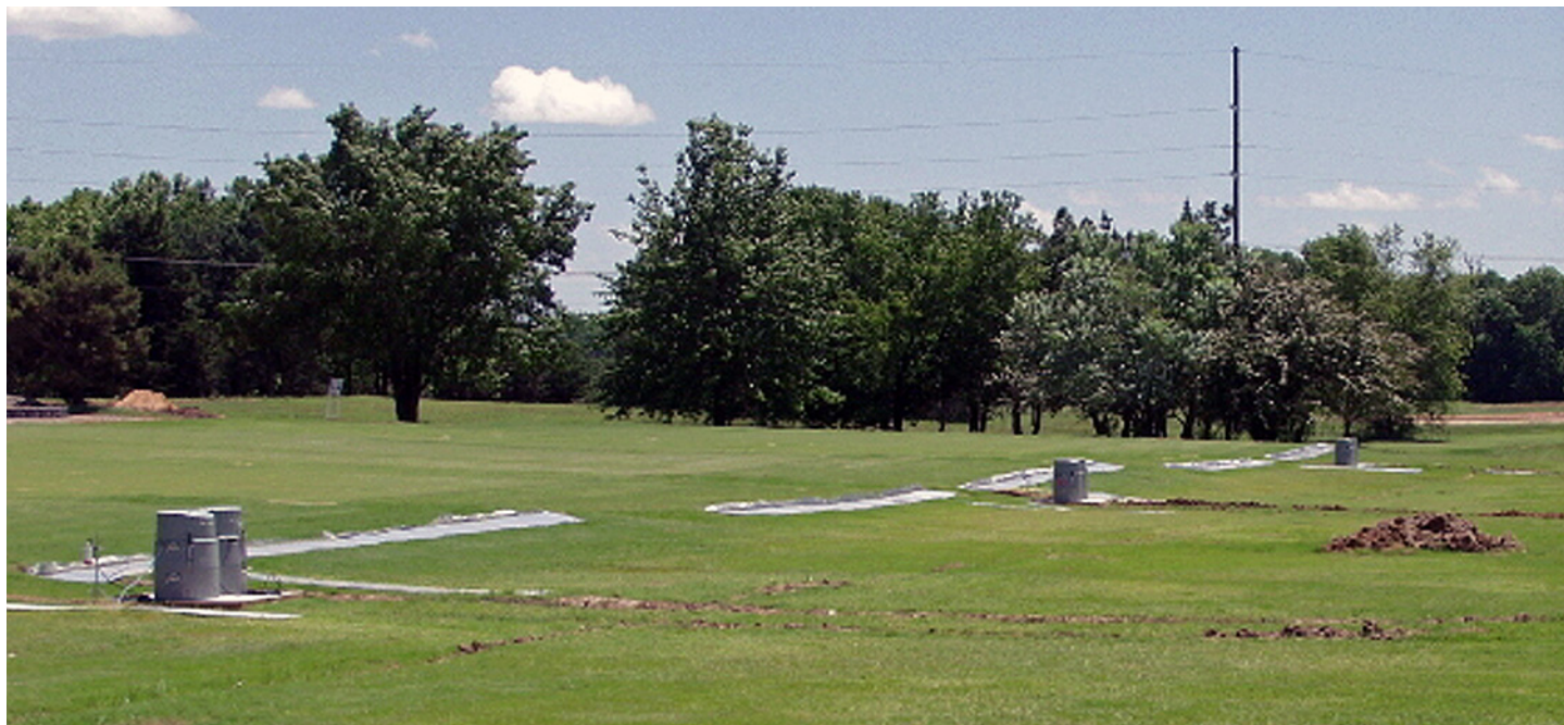
The Oklahoma State University runoff research site. Researchers at Oklahoma State University conducted a five-year study to measure the loss of nitrogen (N) and phosphorus (P) caused by natural rainfall from a common bermudagrass fairway managed with typical fertilization and irrigation practices. Among their findings, in a worst-case scenario during a season of near record rainfall, they estimated that a fairway they studied would lose around 1.3% of the N and 7.7% of the P applied as fertilizer.
