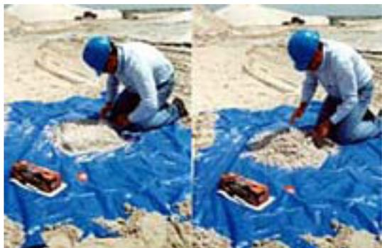
Empty the bucket onto a clean, non-permeable surface. Thoroughly mix the samples together by hand. The combined sample should now be reduced to approximately 1 gallon to be sent into the laboratory. This is accomplished by splitting the sample. The sample should be shaped into a square so that it can be divided into quarters.
