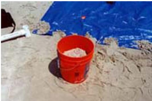
After the eight samples are collected from the 1000-ton pile, the 5-gallon bucket should be about  $\frac{1}{2}$  to  $\frac{2}{3}$  full. (If a stockpile larger than 1000 tons is sampled, the number of samples collected should be increased proportionately. Thus, at least 16 samples should be collected from a 2000-ton pile.)
