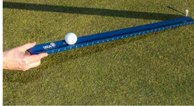
The USGA Stimp meter measures green speed and provides valuable information to assist golf course superintendents.
