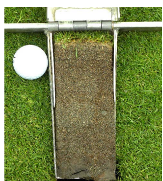
When aeration and topdressing programs properly dilute thatch accumulation, a rootzone free of organic layers is achieved. This soil profile exhibits excellent thatch management and blending of the new rootzone (sand topdressing and organic matter accumulation) with the sand-based construction mixture below.
