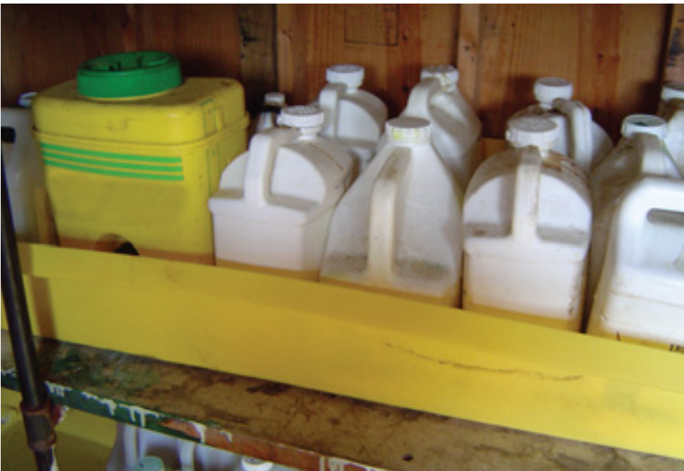
Placing bottles in plastic or metal storage bins is an inexpensive way to create secondary storage.
