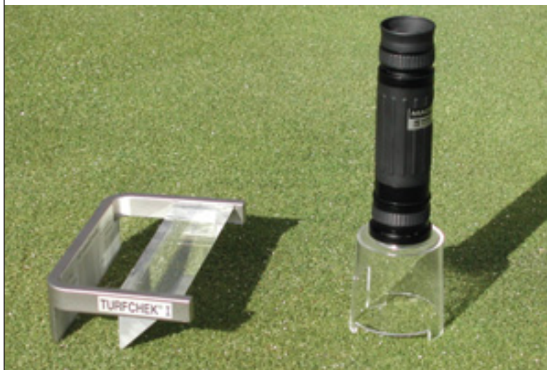
A macroscopic prism gauge and turf gauge are helpful in examining quality of cut and sand incorporation following topdressing.
