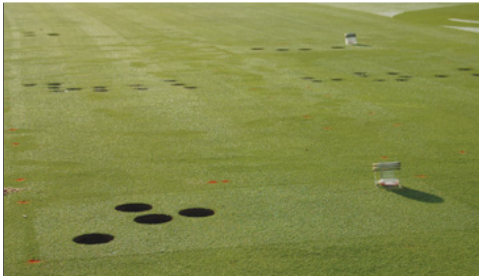
Foliar nitrogen is applied to the putting green turf and an ammonia volatilization trap is installed after application.
