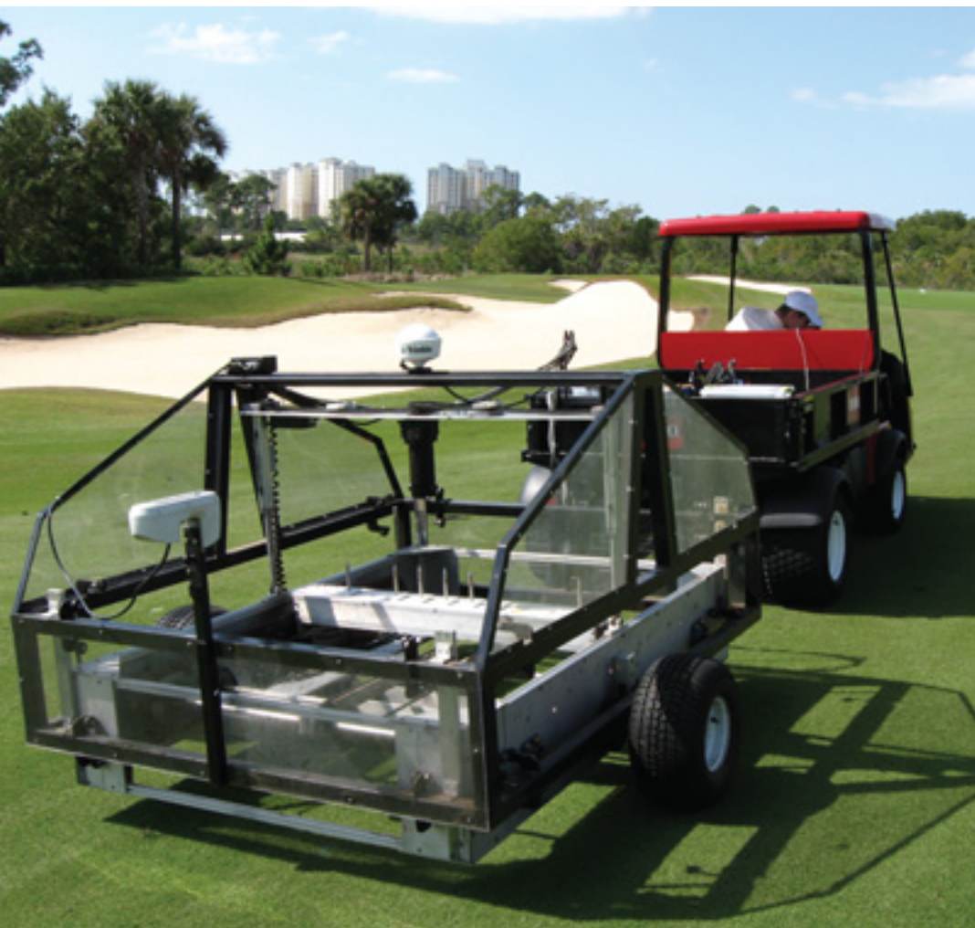
Experimental Salinity Monitoring Device (SMD) conducting salinity mapping of surface salinity, subsurface salinity, and plant NDVI at Old Colliers Golf Club, Naples, Florida. Data are GPS labeled, and the mapping grid is 5 by 10 feet. Photo courtesy of Toro.
