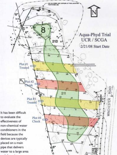
effectiveness of non-chemical water conditioners in the field because the devices are typically placed on a main pipe that delivers water to a large area and there is no option of including a non-treated check area for comparison. A better test would be to include both treated and nontreated areas on a single fairway as noted with this experimental design by Drs. Green and Wu at the SCGA Golf Course.
