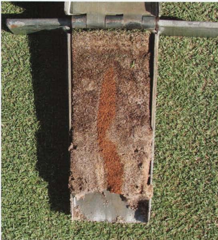
The Drill and Fill aeration machine was first developed by Ray Floyd's father in the early 1970s. It drills 10" to 11" deep and then completely fills the hole with the selected sand or sand/inorganic amendment blend.
