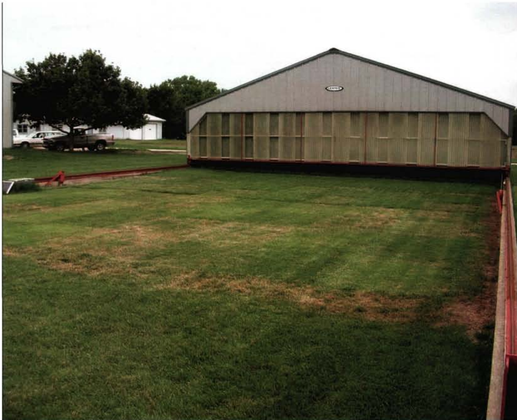
To control water inputs and ensure drought-like conditions, an automated rainout shelter mounted on steel tracks (background) moves to cover plots (foreground) when it rains.
