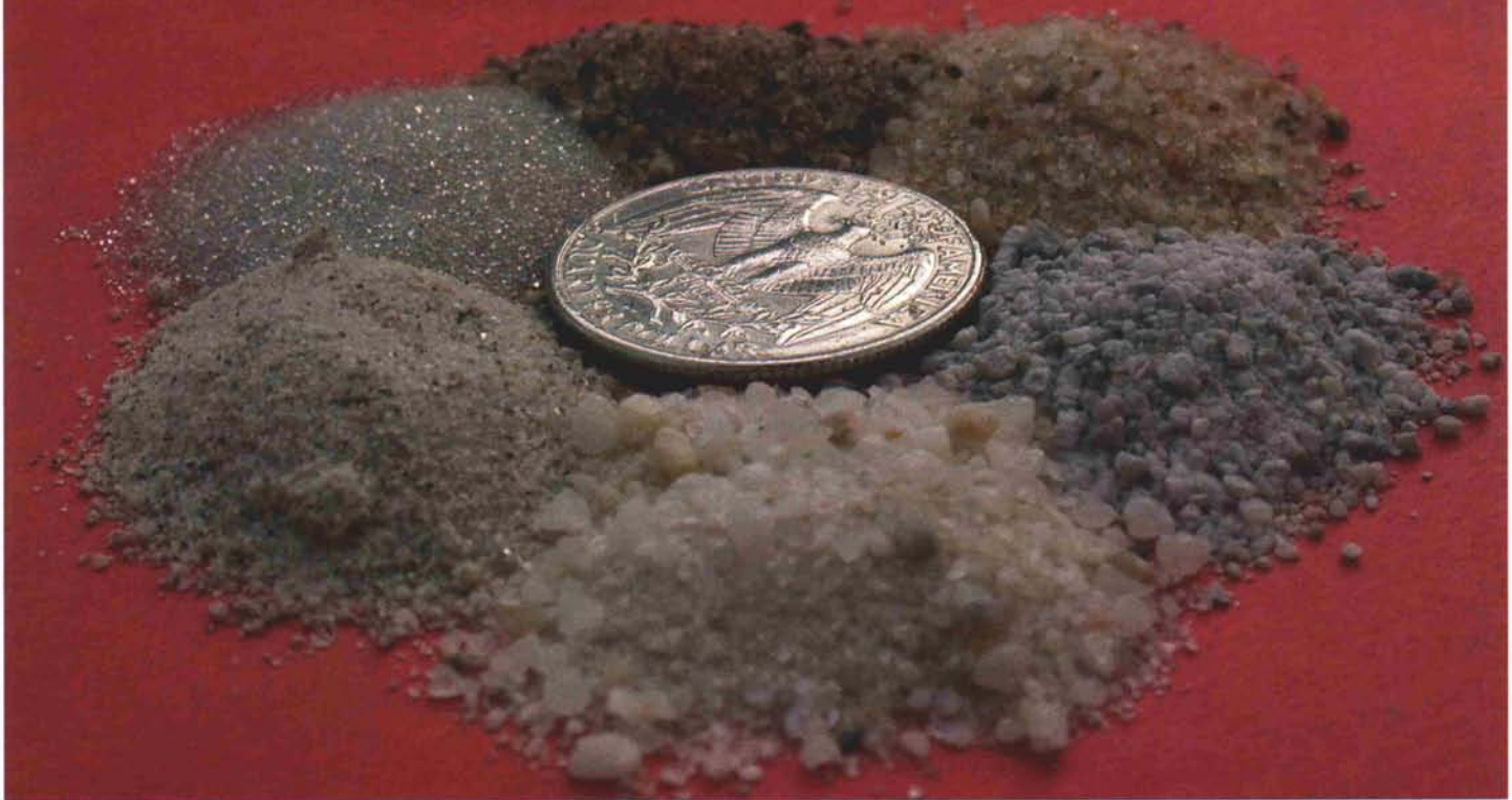
This laboratory study at Purdue University evaluated the physical properties and visual characteristics of more than 20 bunker sand materials. No single sand physical property or combination of properties was able to accurately predict sand firmness or resistance to golf ball penetration.
