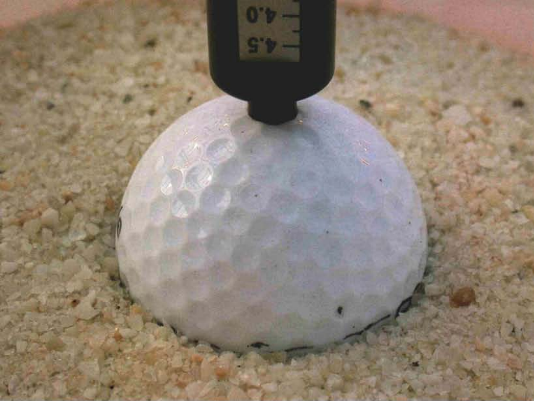
The penetrometer device pictured above is currently the best means to quantify the firmness of bunker sand in the laboratory. The penetrometer device and laboratory test may soon be replaced by a new procedure that will reduce the variability of the current measurement.
