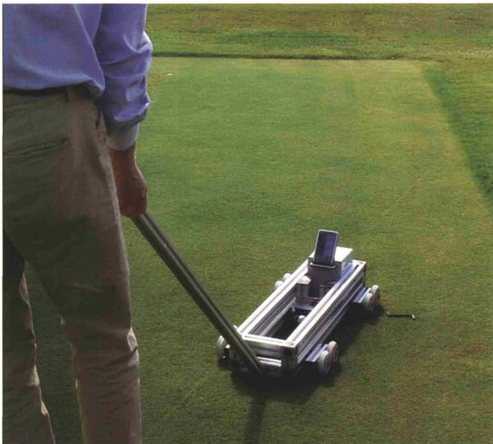
This device, which measures the trueness of a putting surface, will give the superintendent the information he needs to present better surfaces for the golfer.
