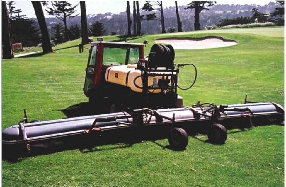
One tool to use as part of best management practices is a hooded sprayer to cut down on spray drift when applying insecticides.
