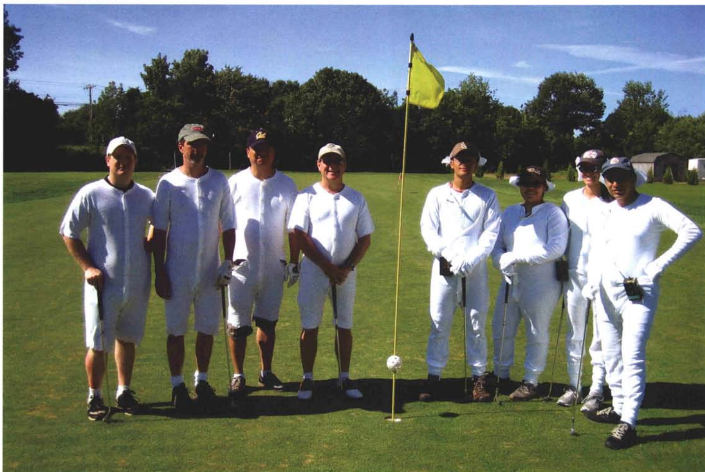
Pesticide exposure was measured by dosimetry and biomonitoring. The dosimetry group (on right) wore full-body cotton suits and personal air samplers. The biomonitoring group (on left) wore matching suits cut to simulate the body coverage of normal golfer attire.
