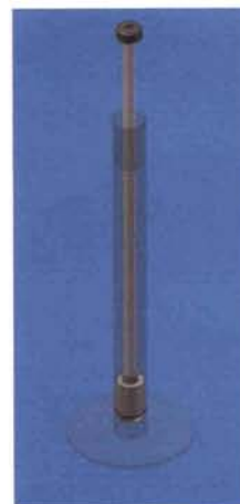
The slide hammer within the tube and its hemispherical face are designed to mimic the energy and momentum of a golf ball. The design provides the same drop height at each test location when the shaft is fully extended.
