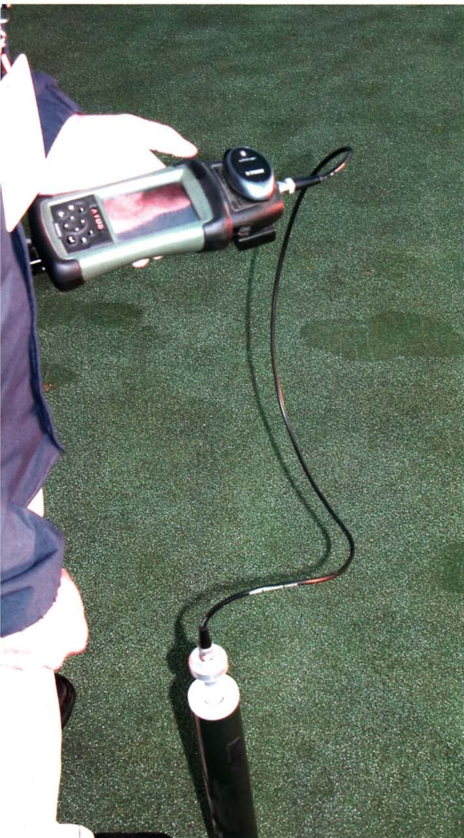
A handheld PC is connected to the slide hammer to record data. The added GPS receiver correlates the location of each data collection drop.
