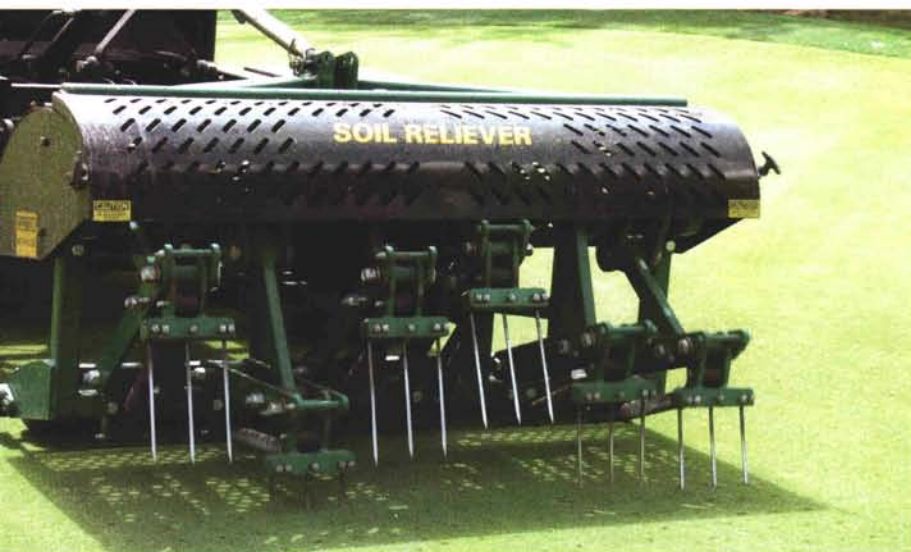
Deep aeration on greens, using \frac{5}{16} " needle tines, has become a popular program to enhance water percolation and allow for the removal of soluble salts from the rootzone.
