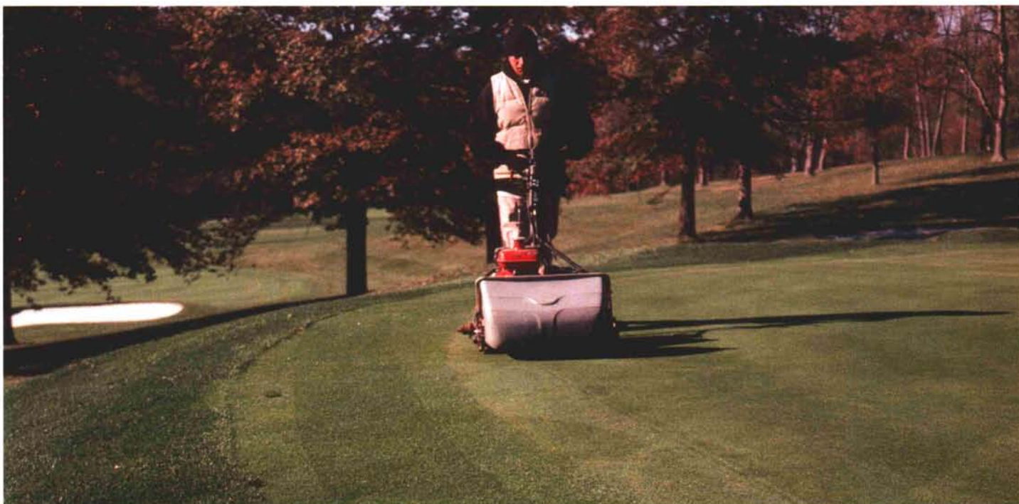
John Shaw instructs his employees to complete the cleanup pass six inches inside of the collar/putting surface interface.
