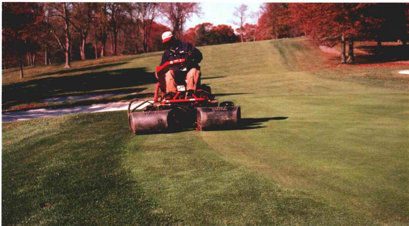
A triplex mower is set up to maintain the collar. One of the cutting heads is set at putting green height. This technique allows the collar to be sustained at two cutting units wide.
