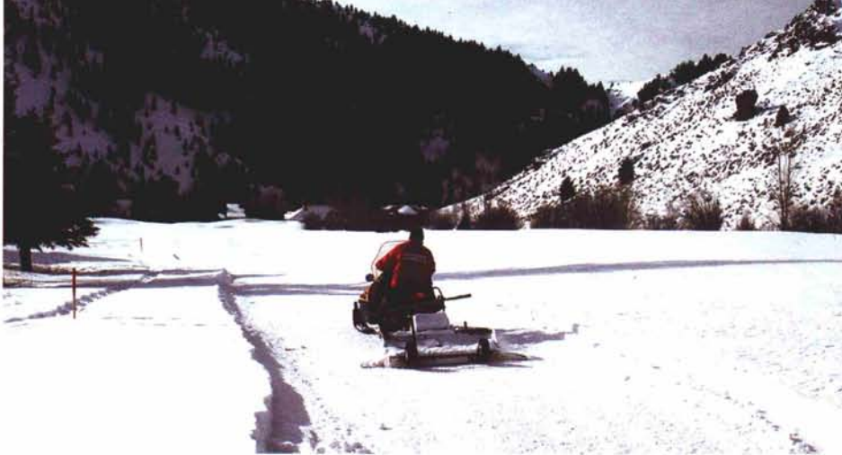
Snow machines with tow-behind grooming attachments are an affordable and efficient method of grooming Nordic ski trails on golf courses.
