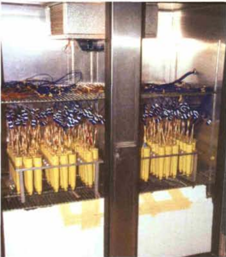
Bermudagrass plants are acclimated to fall-like temperatures, trimmed of top growth, and placed in a programmable freeze chamber to be exposed to sub-freezing temperatures.
