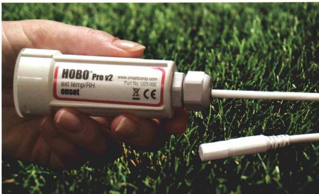
Data logger devices like the one pictured are durable enough for use in the field and will operate effectively for months on their battery source. The device collects and stores large quantities of data that can be transferred to a computer for analysis.
