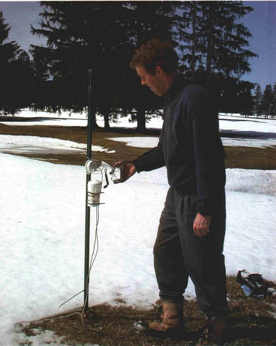
Chris Frielinghaus, superintendent at Glens Falls Country Club, uses a data shuttle device in the field to download temperature data from the data logger to be later transferred to his computer.
