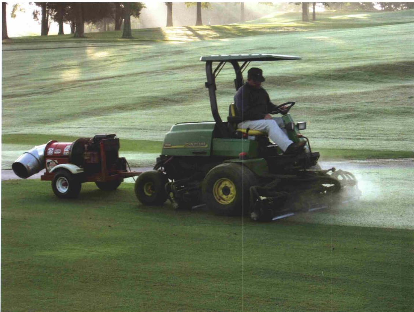
Combining mowing and clipping dispersal allows the staff to get one more job done before play. Best of all, both of these jobs are done with one operator.
