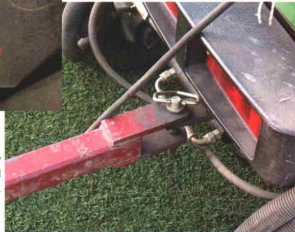
The blower and fairway mower unit are attached via a simple hitch.
