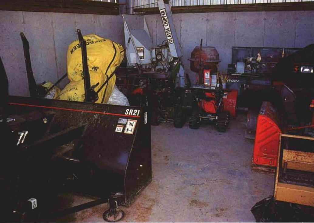
Tractor-mounted snow blowers, walk-behind snow blowers, and green covers are tools commonly used to remove snow from greens and safeguard turf health in the Rocky Mountains.
