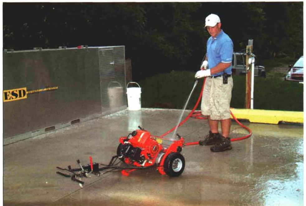
Make sure your chairman knows about your efforts to be a good steward of the environment. Here, clippings and other debris are removed from the wash water and are degraded. The water stays in the system and is recycled.
