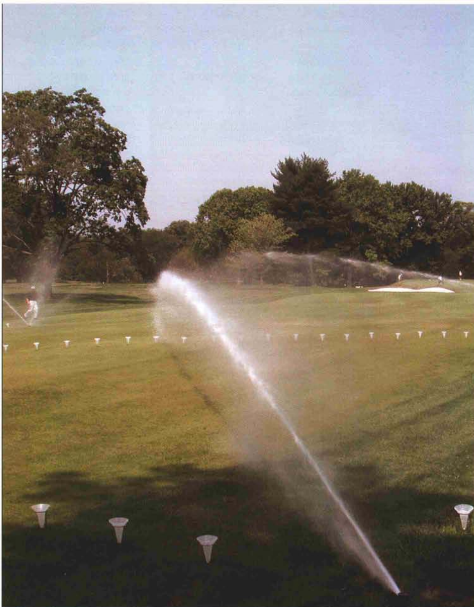
Watching sprinklers function does not tell the complete story. More evaluation, such as using catchment tests, is necessary to accurately characterize performance.
