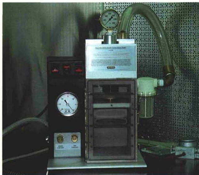
The biolistic gun has been used in the lab to transform turfgrasses. External DNA is coated on the surface of small particles of tungsten and the particles are physically shot into plant cells.
